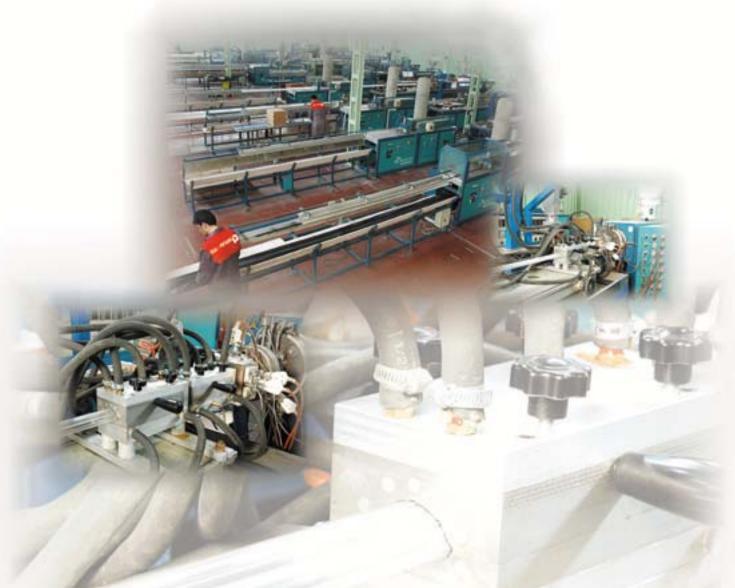
More than a dozen High Tec extrusion lines, single screw and double screw operate to manufacture various sizes of different plastic profiles within tight tolerances. Value added fabrications including drilling, notching, punching, hot stamping, printing, barcode labeling, tape applications and lamination may be applied on profiles if required.
